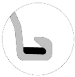
Interlock with bitumen
